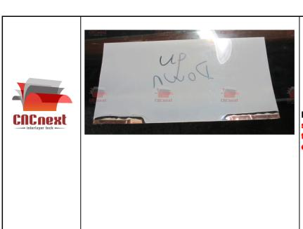
Put the copper tape onto the conductive glue, make sure one copper of one side is longer to be bent on to the other sizde, so we can soldering both electrodes on same side
