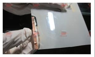
Put the copper tape onto the conductive glue, make sure the copper of one side is longer to be bent on to the other sizde, so we can soldering both electrodes on same side
